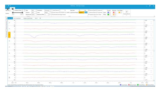
Test traces display of either or both Quad and Phase on all traces.
