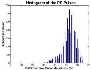
PD generation: Test cell gap 0.05mm recorded in parallel with IEC 60270 system and UHF system
