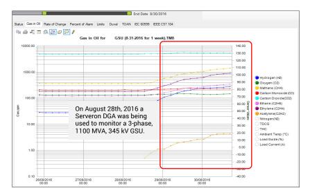
*Figure 1:* TM View Screen showing the time at which gases started to increase. Log Scale is used to best illustrate the very large increase of gases on a single graph
