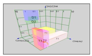
**Figure 2:** Rodgers Ratio indicating condition T3: Thermal Fault 300°C – 700°C
