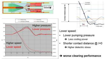
Figure 2- Impact of lower speed on short circuit switching performance. A slower speed results in a smaller mechanical pressure build up in the interrupting chamber. This reduces the blowing pressure at current zero with a consequent reduction of thermal switching capability. Additionally, the contact distance reached for the same arcing time is smaller, which increases the probability of dielectric failure around TRV peak.
