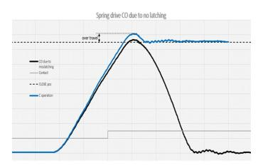
Figure 5 - Travel curve of a circuit breaker with spring operating mechanism. - If the over travel is below the minimum, the latching is not successful and the contacts open again. A Close operation results in a Close-Open sequence.
