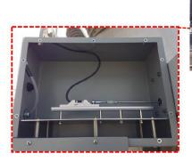
Figure 10 - Linear transducer with linkage
