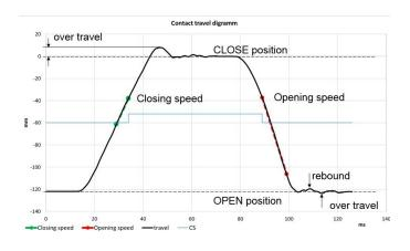
Figure 1 Typical travel curve for a CO operation.
